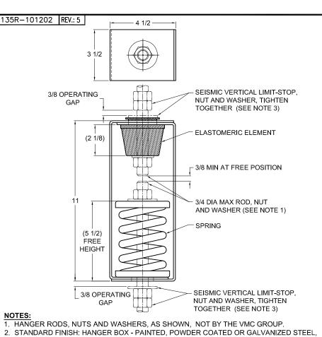
3. SEISMIC VERTICAL LIMIT-STOP HARDWARE REQUIRED FOR SEISMIC APPLICATIONS, NOT BY THE VMC GROUP. INSTALL WASHER .148 THK, MIN, X 2 O.D. MIN, WITH REQUIRED INSIDE DIAMETER TO ACCOMMODATE ROD SIZE IN USE. THIS CAN BE ACCOMPLISHED BY USING A SINGLE WASHER OR BY STACKING NOT MORE
